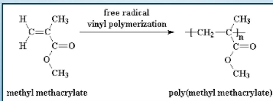
**Properties:** Poly(methyl methacrylate) is a linear thermoplastic, about 70-75% syndiotactic. Due to lack of complete stereoregularity and its bulky groups, it is amorphous. The outstanding property is its optical clarity and lack of color.
