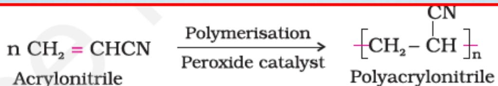
**Properties of acrylic fibers:** The acrylic fibers exhibits the properties of very high strength, stiffness, toughness, abrasion resistance. They are relatively insensitive to moisture, good resistance to stains, chemicals, insects and fungi.
